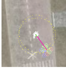
Fig. 6. Flight trajectory (marked in yellow ) of a misconfigured UAV (marked in green ) under RTL mode. The UAV, stuck in a circle around the home location and failed to land, was caused by misconfigured PID parameters.
