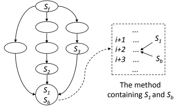
Figure 3. A fragment of a call graph with call paths from the method containing  $S_f$  to the method containing  $S_b$
