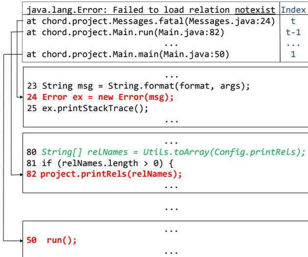
Figure 1. Example showing how developers diagnose a configuration error based on the stack trace. The statements in bold (red) are program points referenced by the stack trace entries. The statement in italic (green) is a read point of a configuration option.
